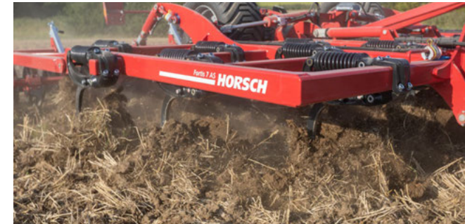
4-bar design for intensive mixing
