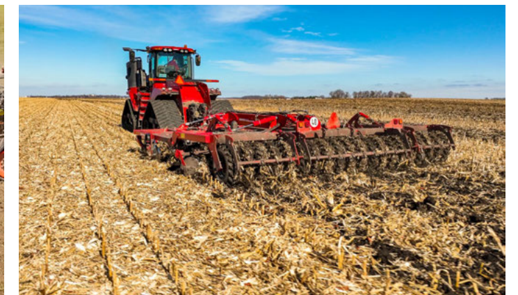
Intensive tillage due to discs and shanks
