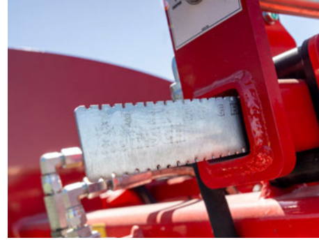
Scale to adjust depth in the back
