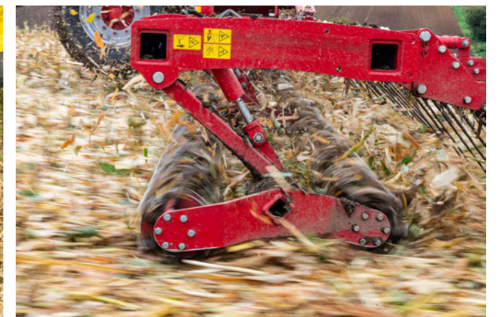
Double knife roller with a theoretical cutting length of 14 cm
