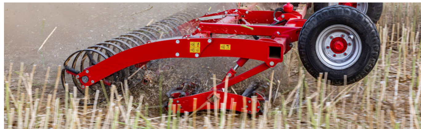
6 Optional with packer for even consolidation
