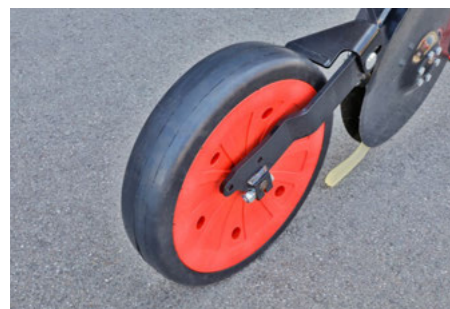
ParaDisc seed coulters – 7 cm wide press wheel
