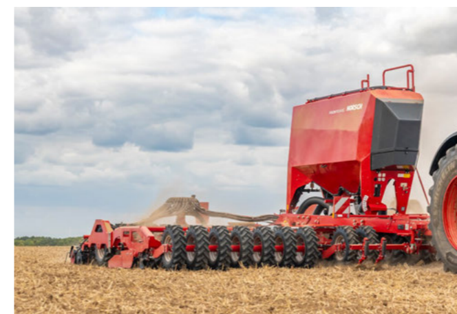
Track eradicator tines to loosen the tractor's track
