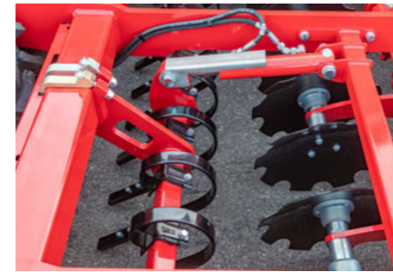
The 1-row Crossbar directly behind the DiscSystem can be adjusted hydraulically .
