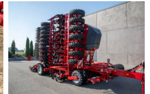
One-side folding of the Pronto 9 DC
