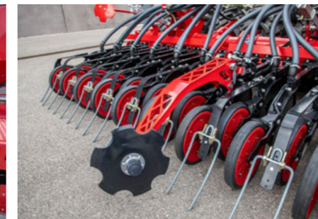
The aggressiveness of the pre-emergence marker is adjusted via a depth stop
