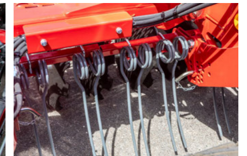
The harrow is placed between the DiscSystem and the tyre packer. The adjustment is carried out mechanically via a hole pattern.
