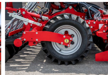
Low horsepower requirement due to large tyre diameter and no scrapers required
