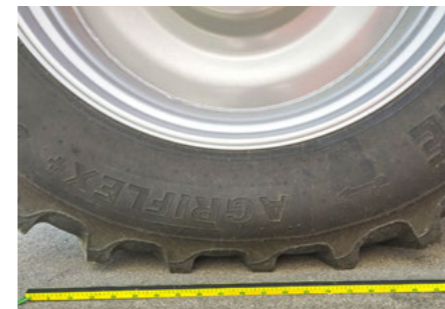
ATP Control – smooth running with a tyre pressure of 2.3 bar
