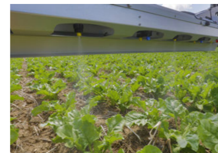
Band spraying is also no problem for a 25 cm spacing
