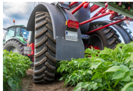
Steering axle with a steering angle of up to 28° even with large tyres
