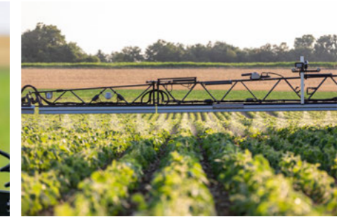
Efficient band application of the nozzle directly above the plant row with optional camera steering
