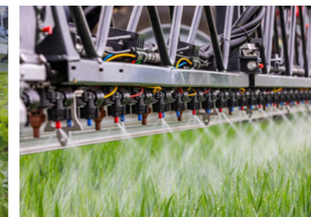
25 cm nozzle layout: more nozzles, more options, e.g., 3D application
