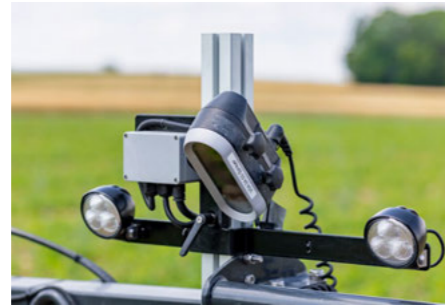
Camera steering CultiCam with light kit for working in difficult lighting conditions
