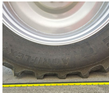
ATP Control – smooth running with a tyre pressure of 2.3 bar
