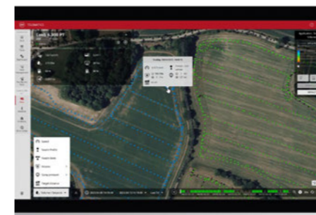
Success factor transparency: position-specific data of all relevant information like error messages, application rate, nozzle status or target area spacing
