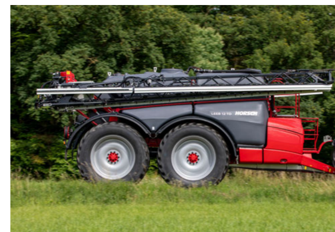
Smooth road holding with tandem axle unit and hydraulic suspension
