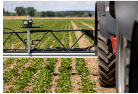
High-precision steering of the trailed sprayer with CultiCam
