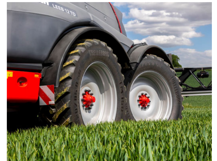
DynamicSteering – intelligent kingpin steering
