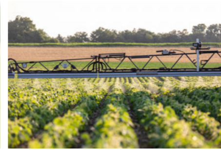
Efficient band application of the nozzle directly above the plant row with optional camera steering
