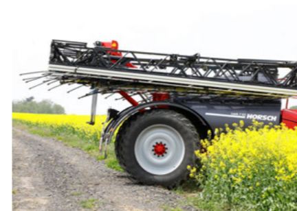
Connect & Fold system – suitable for standard droplegs
