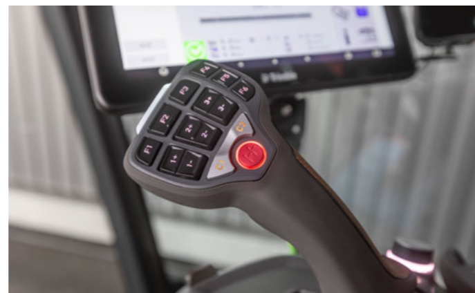
Ergonomic control lever with multiply assignable buttons
