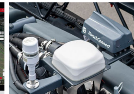
Digital networking with HorschConnect, GPS, and a weather station for optimal adaptation to current environmental conditions
