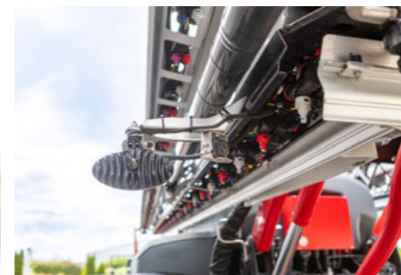
Camera for nozzle monitoring on the NightLight holder
