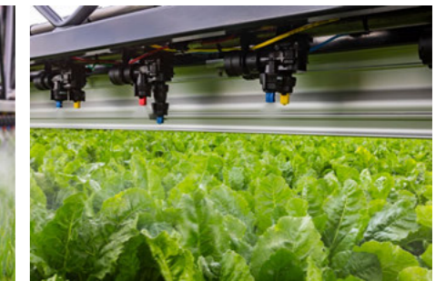
Pneumatic nozzle control 2-2 with 3D application
