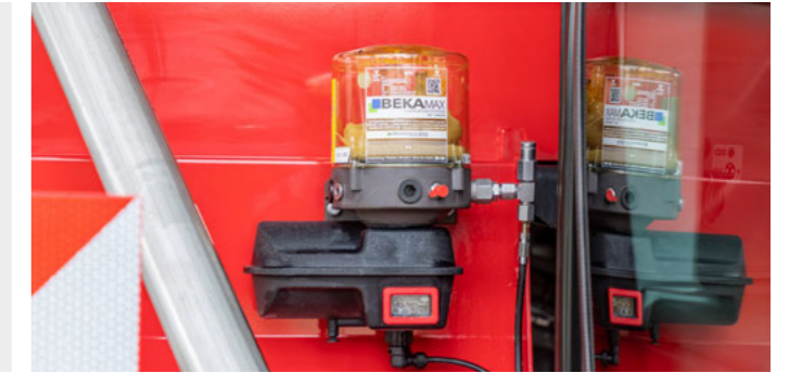
Tank of the central lubrication unit
