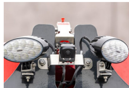
Rear view camera for monitoring the area behind the vehicle
