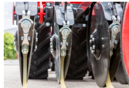
The movable scraper ensures a high self-cleaning effect in wet conditions
