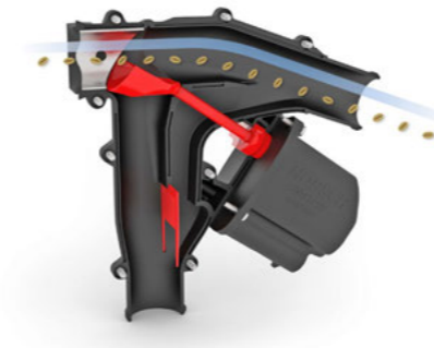
RowControl flap open: seed is transported to the coulter
