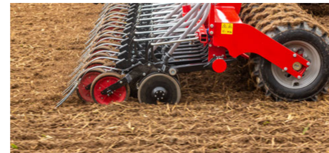
Coulters pressure up to 200 kg is possible
