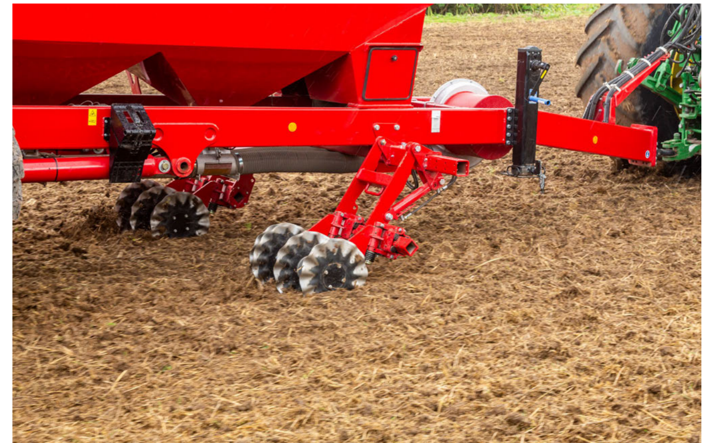
Loosening compacted soil in the tractor track
