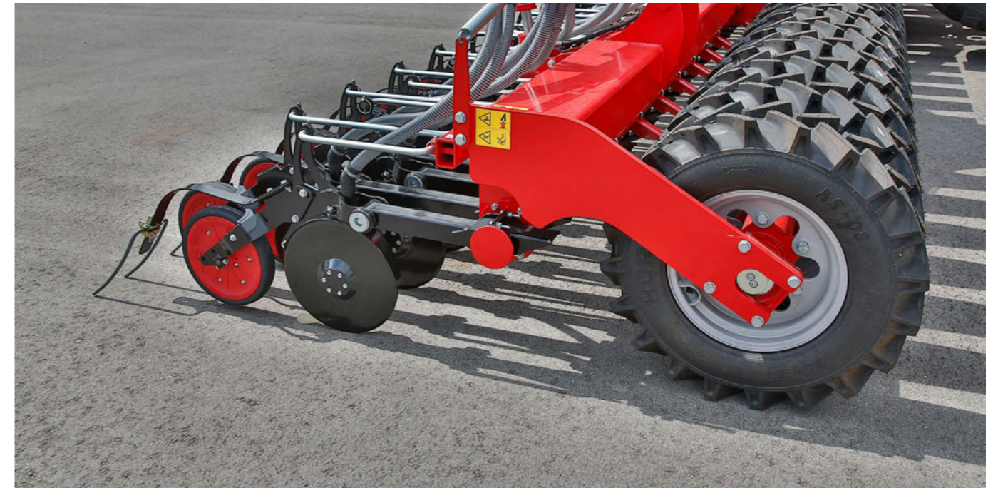
PowerDisc seed coulters – parallel-controlled double disc coulters
