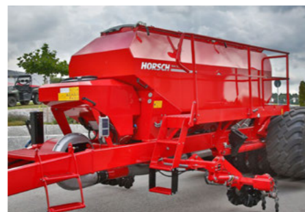
Optional microgranular unit for the easy and safe application of microgranular compounds
