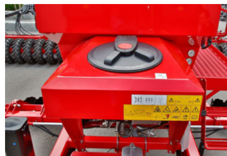
The microgranular unit allows for simultaneously transporting and independently metering 3 components
