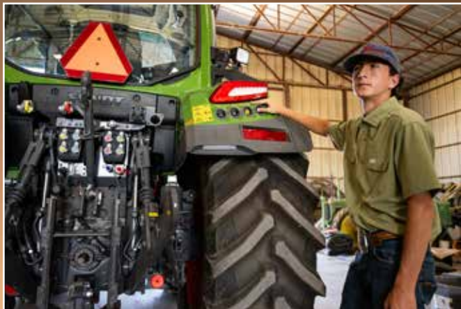
External controls on both rear fenders allow convenient operation of the power lift and actuation of the PTO and hydraulic valves.
